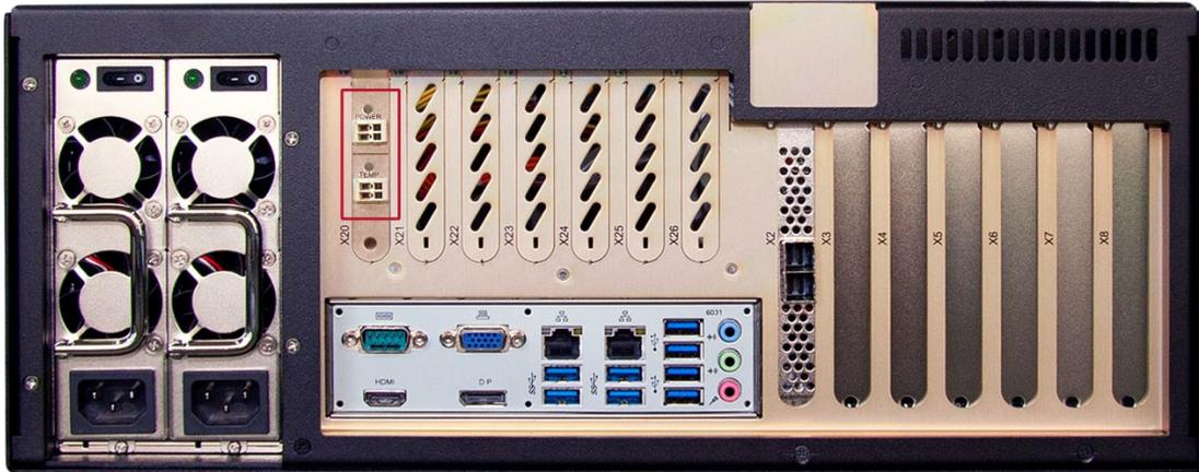
ibaOut-Temp card installed illustrated by ibaRackline-PC
