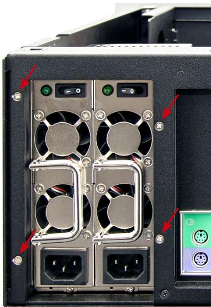
3. Loosen both screws inside, which are used to fix the power supply unit inside the housing.
