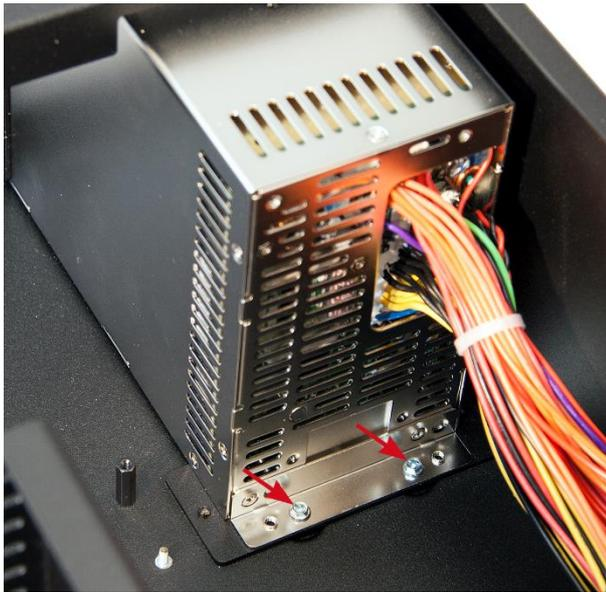
4. Loosen 2 screws each on the left and the right side, which are used to fix the bar (1) and remove the bar.
