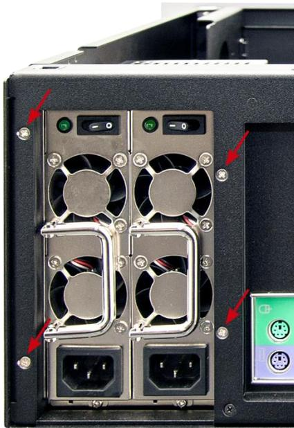
3. Loosen both screws inside, which are used to fix the power supply unit inside the housing.
