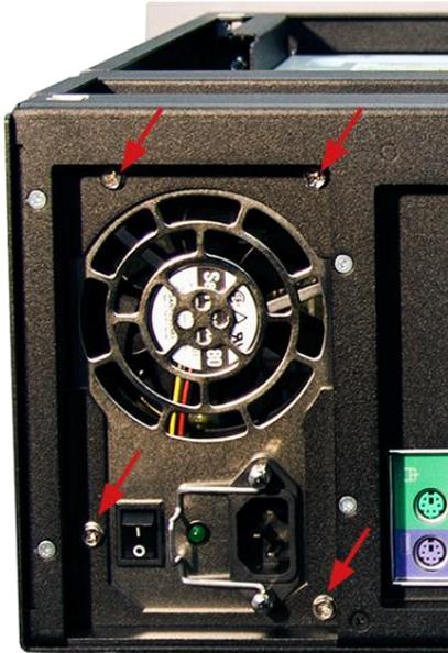
2. Loosen 2 screws each on the left and the right side, which are used to fix the bar (1) and remove the bar.
