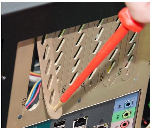
2. Loosen the screws in the openings above the slots.
