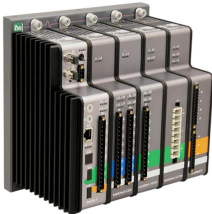
Figure 1: ibaCMU-S with 4 I/O modules
